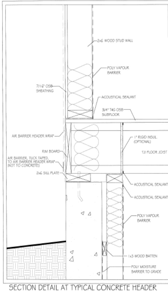
Poly wrap is sealed to poly strip behind wall with acoustic sealant
