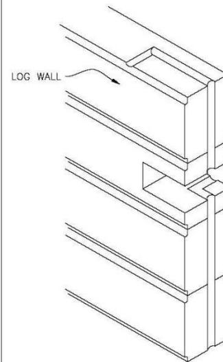
A WIRING CHANNEL MUST BE ROUTERED BESIDE THE HARDWOOD DOWEL AT THE SIDE OF A DOOR. HORIZONTAL DRILLING IS THEN DONE TO POSITION SWITCHES AND LIGHTS WHERE DESIRED. THE BOTTOM ACCES MUST BE DRILLED ON SITE AS WELL. CARE MUST BE TAKEN WHEN INSTALLING THE DOOR FRAME SO THAT NO SCREWS OR NAILS HIT THE WIRING.
