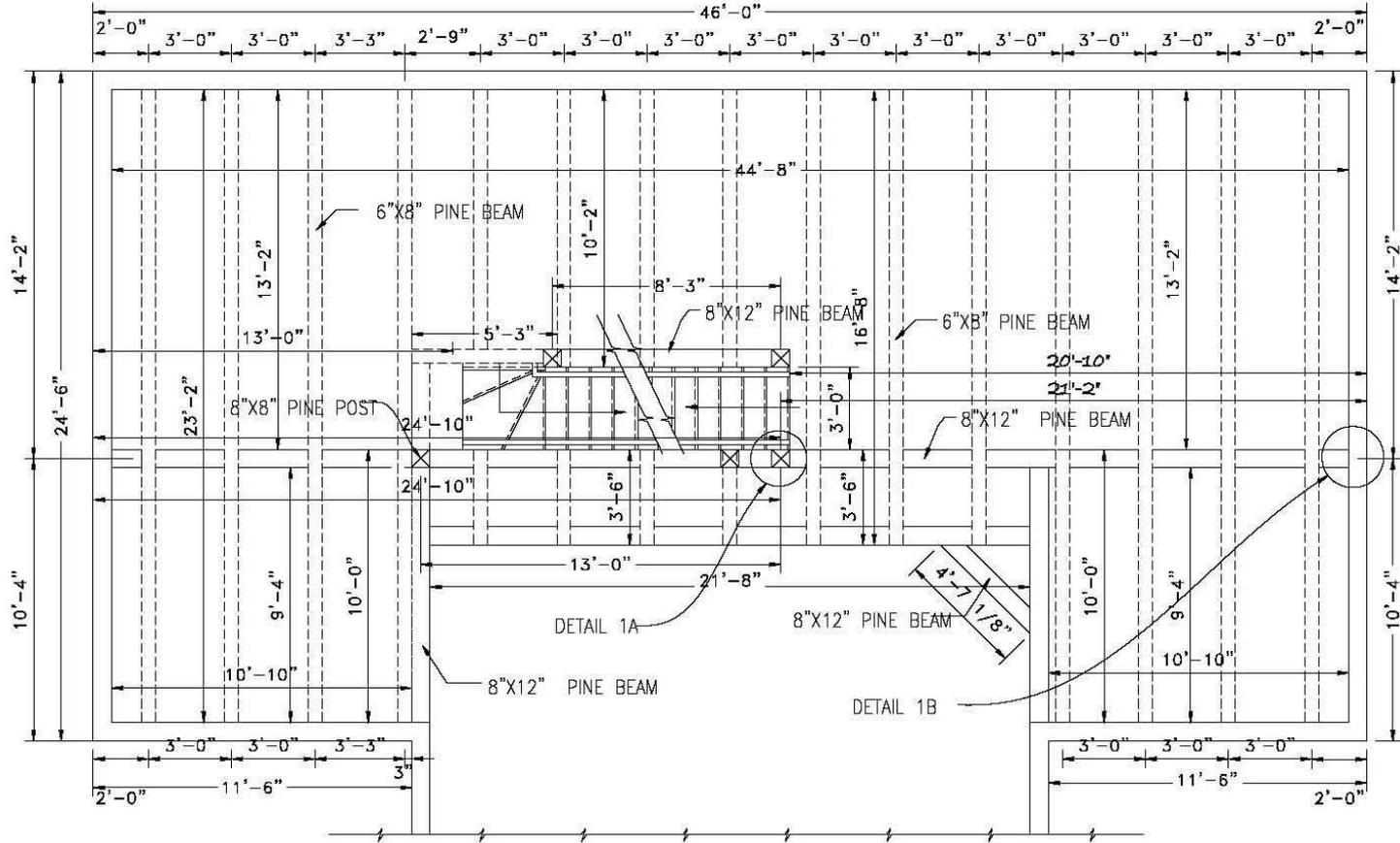
TYPICAL POST AND BEAM FLOOR STRUCTURE
