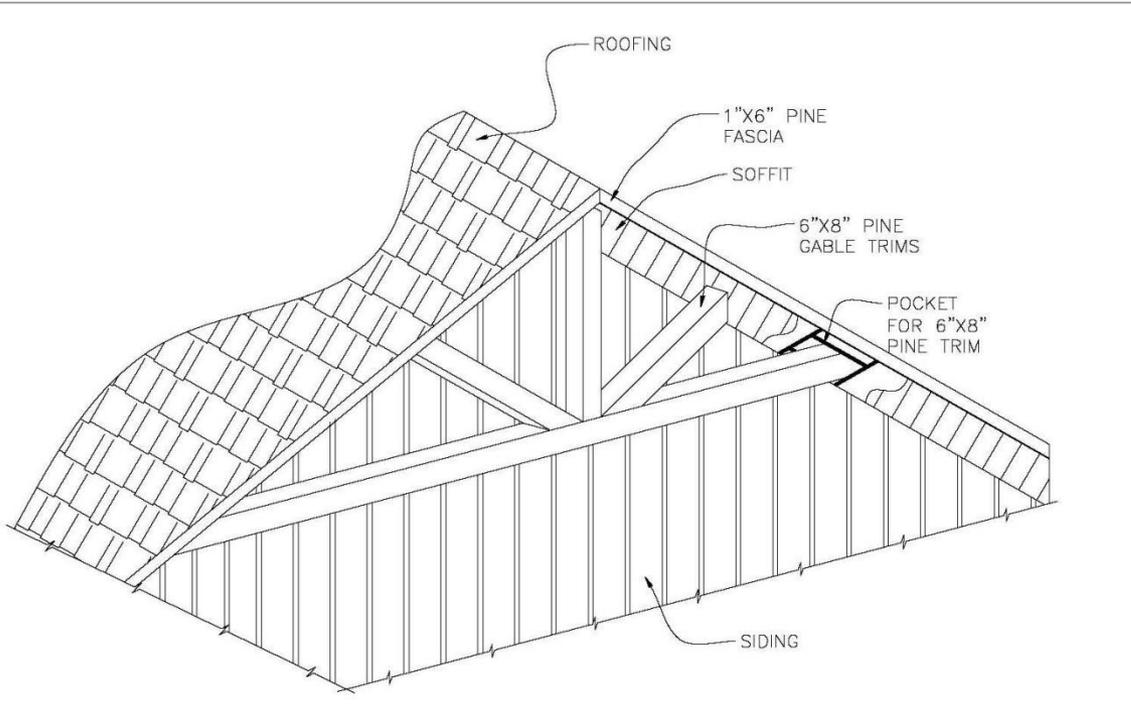
PINE GABLE TRIMS ARE USUALLY CONSTRUCTED OF 6"X8" PINE MATERIALS. THE PIECES MUST BE CUT TO THE PROPER LENGTH ON THE JOBSITE. A POCKET MUST BE CREATED IN THE SOFFIT WHICH THE MEMBERS OF THE BEAM TRUSS CAN BE NAILED. THE BOTTOM CHORD AND THE VERTICAL MEMBER WILL BE NOTCHED, AND CAN BE SPIKED TOGETHER FROM BEHIND. THE DIAGONAL MEMBERS MUST BE ANGLE-CUT TO FIT BETWEEN THE BOTTOM AND THE VERTICAL CHORDS. THEY CAN BE HELD IN PLACE WITH SPIKES.
