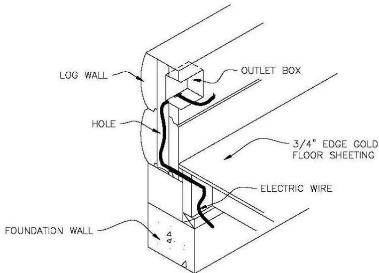
THE STANDARD OUTLET IS TO BE DRILLED UP 2 OR 2-1/2 LOGS. A 1-3/8" HOLE IS TO BE DRILLED AT THE BOTTOM AND WHERE THE OUTLET BOX IS TO BE MORTISED IN. WHEN THE LOG WALL SITS ON THE SUBFLOOR, THE BOTTOM HORIZONTAL 1-3/8" HOLE WILL NOT BE DRILLED. WHEN THERE IS NO SUBFLOOR, (GARAGE ...), THE HOLE WILL BE DRILLED DOWN 88" FROM THE TOP AND MARKED WITH A PENCIL. OVER COUNTERTOPS, THE HOLES WILL BE DRILLED UP TO 55" AND MARKED WITH A PENCIL.
