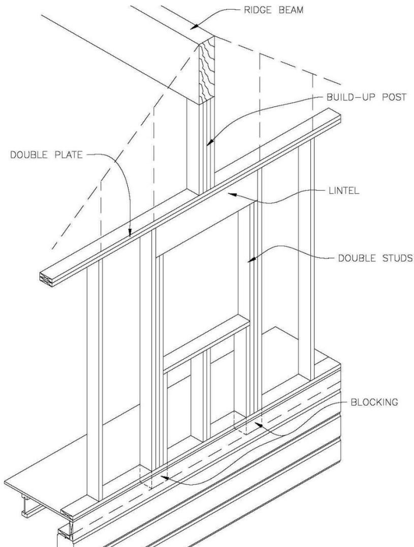
WHEN A RIDGE BEAM FALLS OVER A WINDOW, A PRE-ENGINEERED LAMINATED LINTEL MAY BE REQUIRED. THE LINTEL WILL BE SUPPORTED ON EITHER SIDE OF THE WINDOW WITH DOUBLE STUDS. BLOCKING MUST BE INSTALLED BELOW THE POSTS, IN THE FLOOR, TO TRANSFER THE LOAD TO THE LOG WALL. A BUILT-UP POST IS REQUIRED BETWEEN THE LINTEL AND THE RIDGE BEAM. IT WILL CONSIST OF AS MANY STUDS AS REQUIRED TO MATCH OR EXCEED THE WIDTH OF THE RIDGE BEAM.
