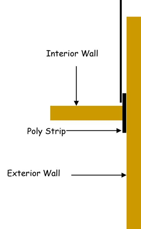
**Interior to Exterior Wall Connection, overhead view**
