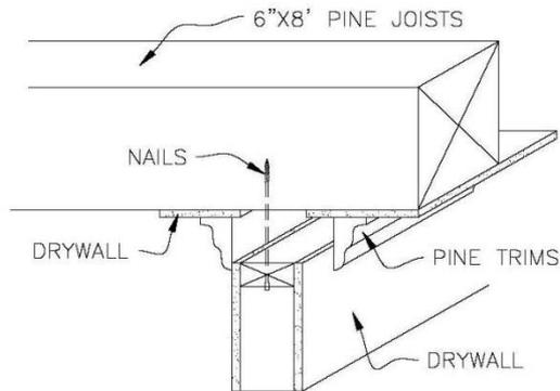
FOR A LOG BUILDING, A 2" ALLOWANCE FOR LOG SETTLEMENT MUST BE LEFT OVER SINGLE TOP PLATE OF PARTION INTERIOR WALLS. THE PARTITIONS ARE HELD IN PLACE BY 5" TO 6" NAILS OR SPIKES @ 6'-0" O/C, NAILED IN TOP PLATE INTO 2"x4" NAILERS OR CEILING MEMEBERS. THE MOULDINGS ARE NAILED ON THE FINISH CEILING FINISHING ONLY. WHEN THE HOUSE SETTLES, THE MOULDING WILL SLIDE DOWN THE SURFACE OF THE WALL.
