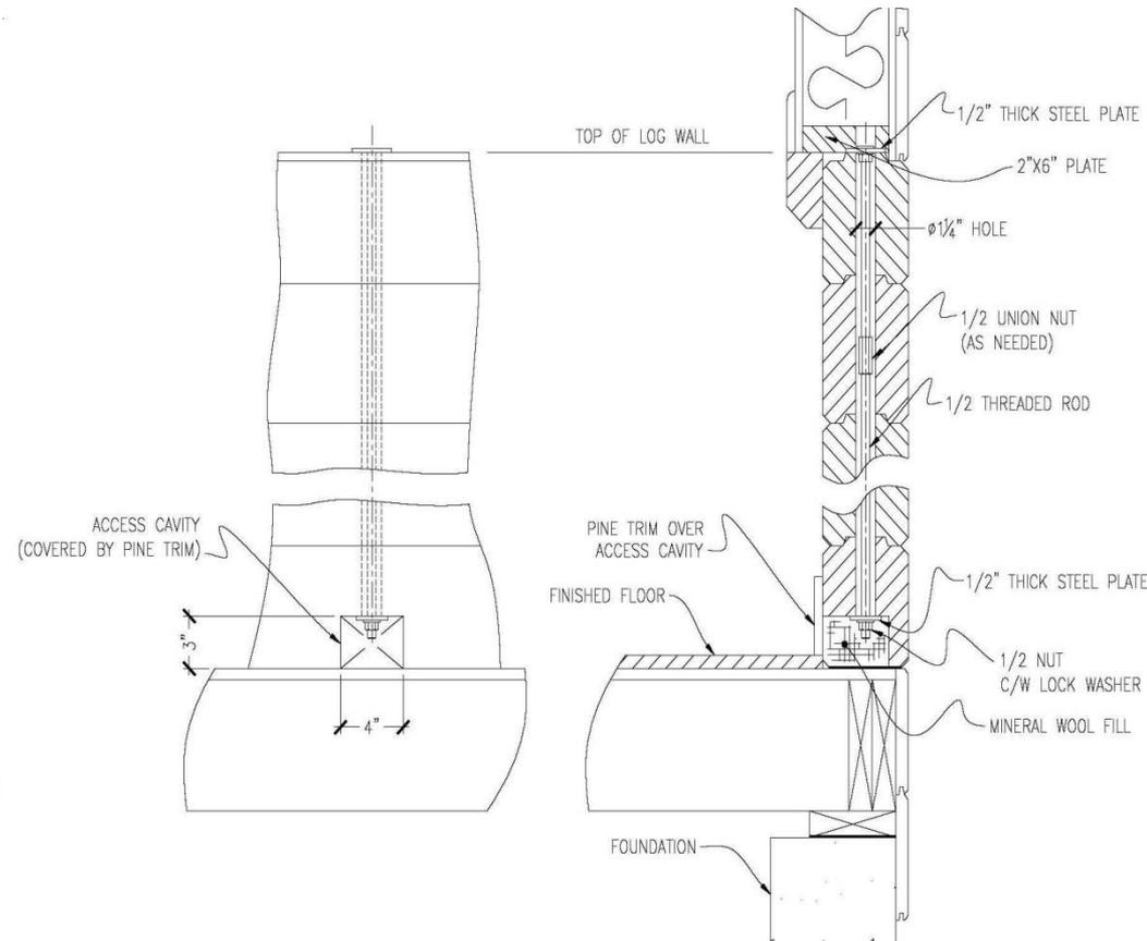
The butt joints overlap for lag bolts has to be a minimum of 24" between rows and thru-bolt system.
