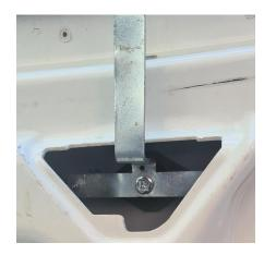
Remove the clamp or tape on the rods
