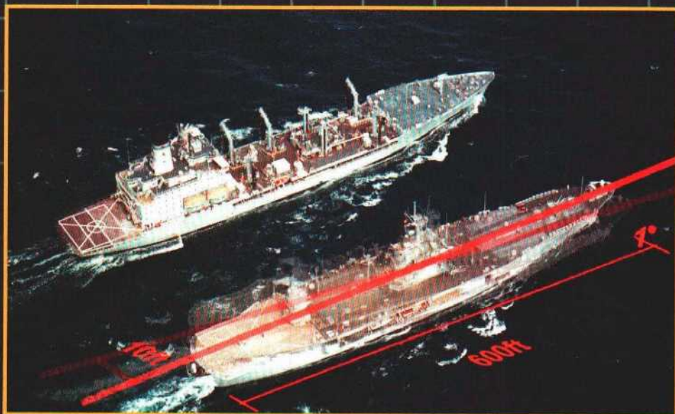
▲ The Amphibious Command Ship (right) has an overall length of approximately 600ft. A 1 degree starboard course change swings the stern toward the guide ship by at least 10 feet, the decrease in pressure due to water moving faster through a narrower opening could make steering more difficult.
