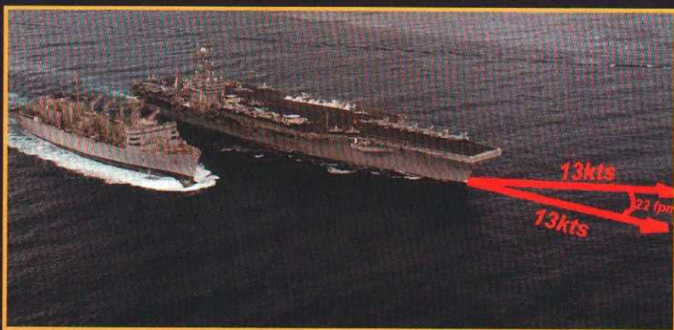
▲ Applying the radian rule to speed vectors, we see a 1 degree course change at 13 knots during calm weather conditions causes the ship to open at 20 feet per minute.
