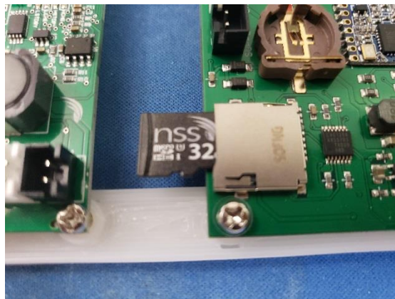
Figure 2: Detail showing the MicroSD card slot and how to insert the card.
