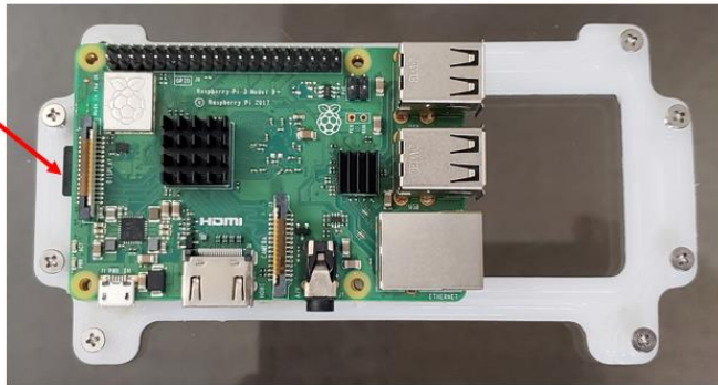
Figure 2: Installation of the Raspberry Pi (not included) on the device chassis and positioning of the Micro SD card.
