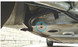
3. Bolt on one of the pucks orientated with the centre of the puck towards the centre of the car along the lateral support (in-line with the other bolts) with the nut, bolt and washer supplied.
