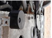
4. Repeat on the opposite side and take a measurement from the under tray fixing or similar to the centre of the puck (this is to be able to get the sticker in the correct position). In my case it was approx. 93mm.
