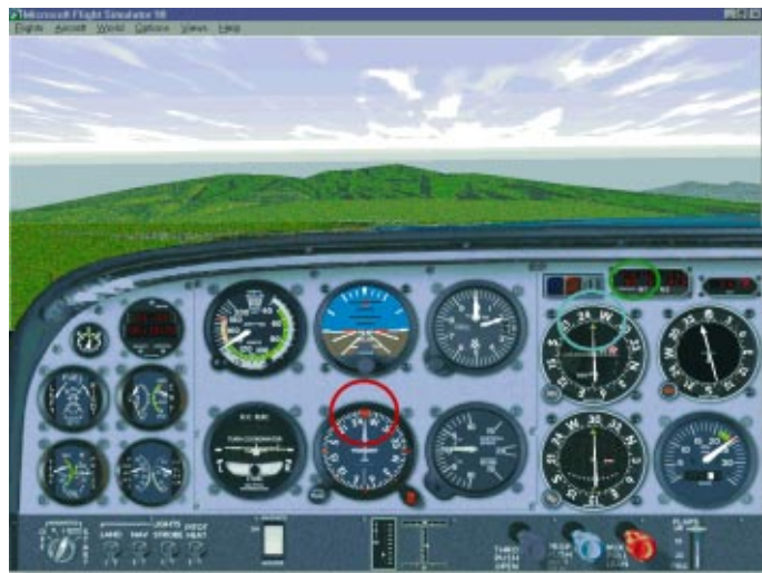
Heading 255° (red) tracking inbound 253° (blue) with 3.4 miles to run (green).
