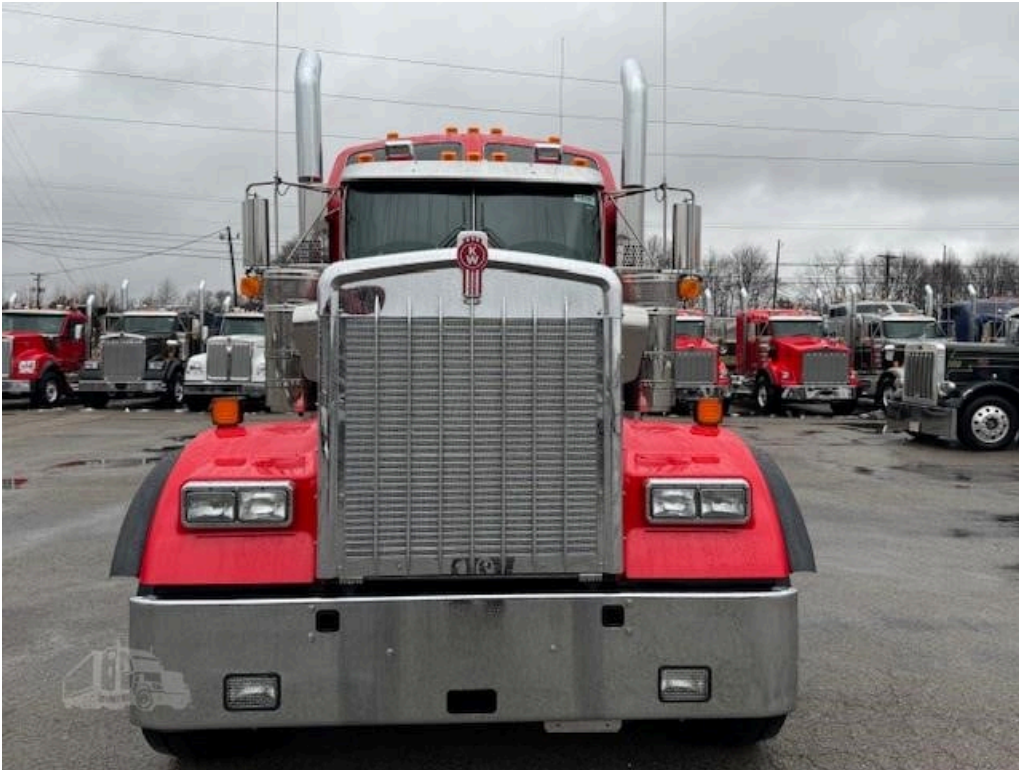
Kenworth W900B with Cummins X15 605hp/2050 Torque w/4 Speed Auxiliary Transmission Spicer TTC AP01750-4C air shift, 22.5K Nonsteer Pusher axle, 52K Neway Suspension
