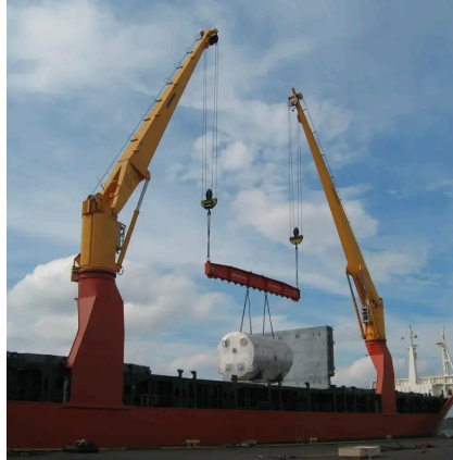
LIEBHERR LS-C 100 TON SHIP CRANES
