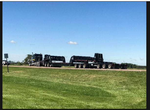
2025 TRAIL KING EXPANDING PERIMETER FRAME TK150 TRAILER Tare Weight – 55,000 lbs. Well Length – 80' Well Width – 12' to 20' Well Ground Clearance – 6'' to 30''
