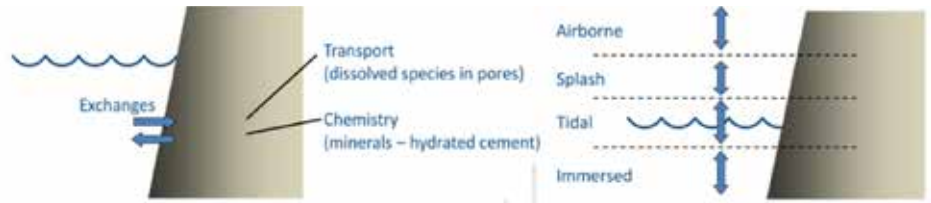
Fig. 1-a) Exchanges of chemical species through the transport process; 1-b) Exposure conditions for marine structures
