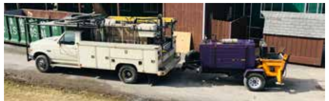
Shotcrete Setup: 1998 REED M40, 2001 Compair 200 CFM, 1993 Ford F-Super Duty
