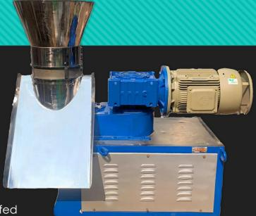
**Basket Extruder** materials are gravity fed up into the granulator and are wiped through SS perforated screens by extrusion blades creating cylindrical extrudates of controlled diameter with Adjustable RPM of Motor Contact us today to learn more about how we can meet your specific needs.
