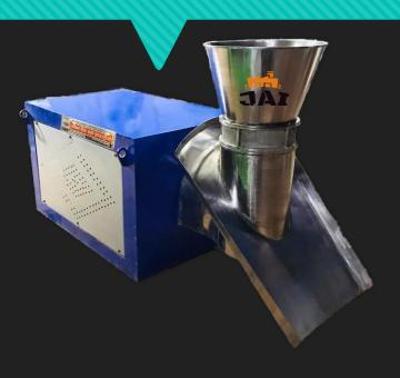
Basket Extruder materials are gravity fed up into the granulator and are wiped through SS perforated screens by extrusion blades creating cylindrical extrudates of controlled diameter. Contact us today to learn more about how we can meet your specific needs.
