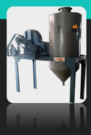
Air Pollution Controller are a series of devices that work to prevent a variety of different pollutants, both gaseous and solid, from entering the atmosphere primarily out of industrial smokestacks. It have an vacuum turbine which sucks pollutants air from workspace and release purify in atmosphere. Contact us today to learn more about how we can meet your specific needs.
