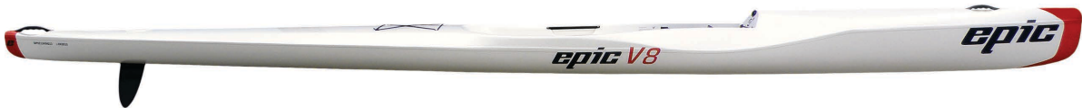
V8 Length 5.48 m • Width 54 cm • Depth 33 cm • Weight (Elite 10.4kg - Ultra 12.5kg - Performance 16kg)
