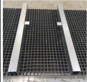
4. When brackets are in place, locate the beams ready for the claws to be fixed. The same brackets are used to fix to walls or support plates using concrete bolts or set screws as per support beam datasheet.
