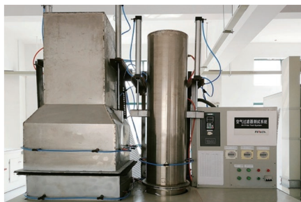
Air filtration testing system
