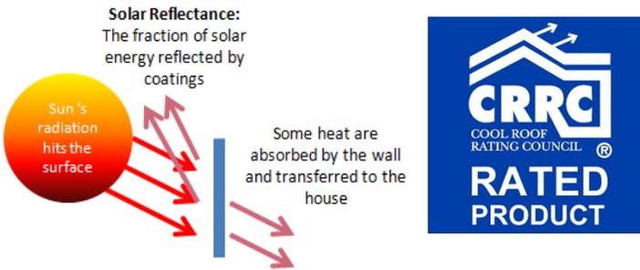
**MS-Thermashield is CRRC Rated with Solar Reflectivity of 0.84, Thermal Emittance of 0.90 and SRI of 106.**
