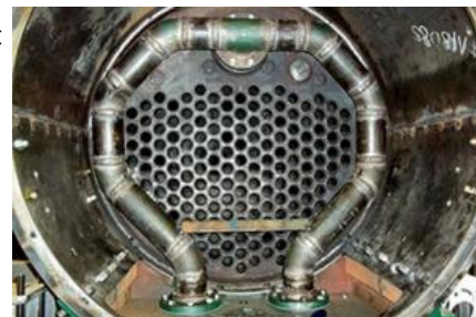
This photo shows the branch pipe header of the York locomotive, which carries steam to power the locomotive. COURTESY OF KLOKE LOCOMOTIVE WORKS
