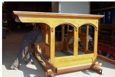
The York locomotive's cab, crafted by Howard Thomas of white oak wood. It took 15 months to build. COURTESY OF KLOKE LOCOMOTIVE WORKS
