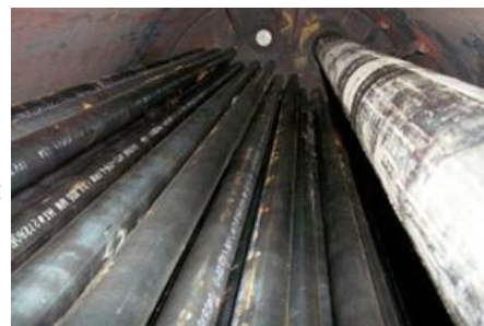
This photo shows the many flues inside the boiler of the York locomotive. Hot gases from the firebox pass through these pipes, which boil the water that fills the boiler. COURTESY OF KLOKE LOCOMOTIVE WORKS
