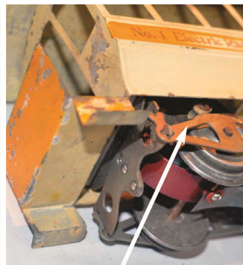
A rubber grommet on each end of the armature shaft presses against a drive wheel.
