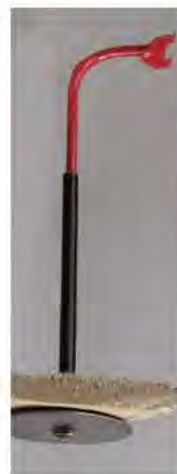
The monorail came with red track supporters which fasten into cast iron bases. The cast iron bases were not used. Threaded lamp pipes raised the red track supporters. The black painted lamp pipes were fastened to the Homasote with large washers and nuts. The pipe section to the left is 7 inches long, much shorter than the 26 inch sections actually used.
