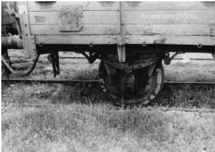
A view of one of the journal boxes on an axle is shown below.
