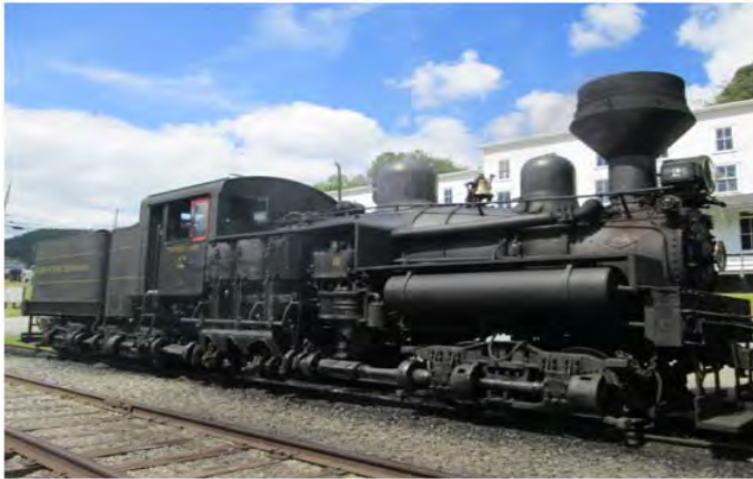
Cass Scenic Railway Shay engine #2 built in 1928. Note all wheels are geared.
