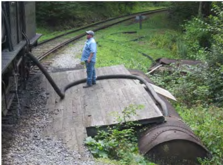
Taking on fresh stream water stored in an old Shay boiler.
