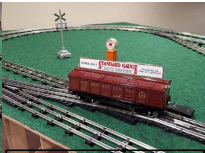
#4 switches provide a smooth transition between loops. Switches are huge, back-to-back length = 44 1/4"
