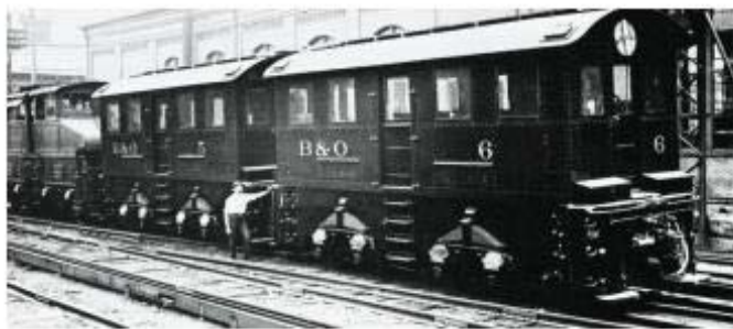
B & O No. 5 and No. 6 General Electric tunnel locomotives. Photograph from B & O Power, 1829-1964 by Sagle and Stauffer, used with permission.
