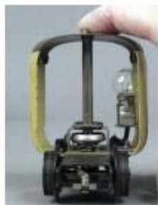
Left, 752 vestibule end view with control rod being pressed downward to enable coupling (or uncoupling) the cars. Right, side view of 752 vestibule attached to 754 Observation.
