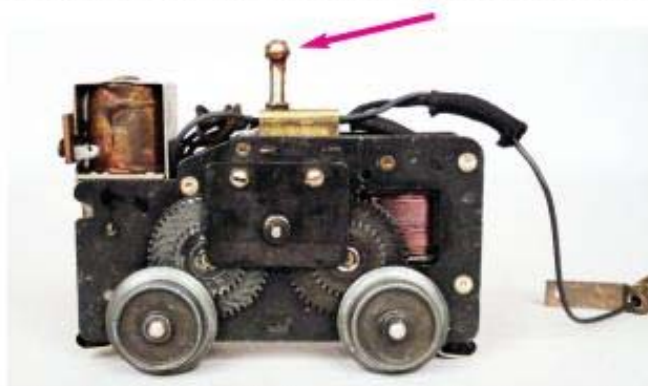
Fastened to the No. 752E motor is a ball (red arrow) which fits into a slot in the casting roof.
