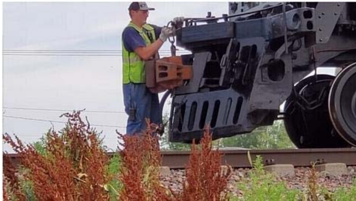
A crewman muscles 4014's front coupler into position and opens the knuckle.
