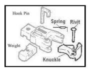
American Flyer's knuckle was held in place just like Lionel's with a rivet and a spring to assist in opening it. American Flyer used a hook pin attached to a weight that, when pushed *up* would release the knuckle. The pin was held down by *gravity*.
