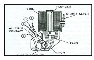
and the pawl would index a small drum on an *horizontal* axis with teeth in the *center* of the drum The pawl would drop down *by gravity* when power was taken off the tracks. In each of the positions, contact strips on the drum would make different contacts with the "multiple contact" fingers that had wires going to the various terminals of the motor.
