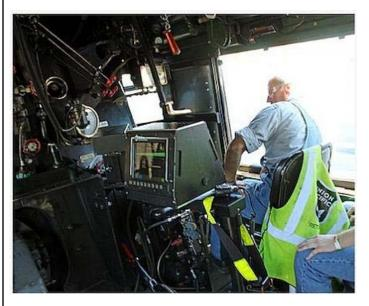
Ed Dickens, manager of Union Pacific's heritage operations, glances at the PTC screen mounted in the cab of Big Boy No. 4014. The screen is situated so both engineer and fireman can read it while the locomotive is in operation. The new system, recently installed, will allow operation without a trailing diesel locomotive. Bob Lettenberger
