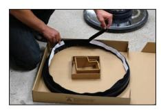
2. Remove VELCRO® with white adhesive backing from the inside of the dust skirt. Then remove the backing from the VELCRO® exposing the adhesive for attaching to the housing of floor machine.
