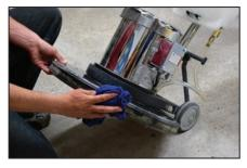
1. Clean the floor machine housing (bumper) of any residual dirt and debris. To be sure the surface is completely clean, use a clean cloth and any household cleaner or alcohol.
