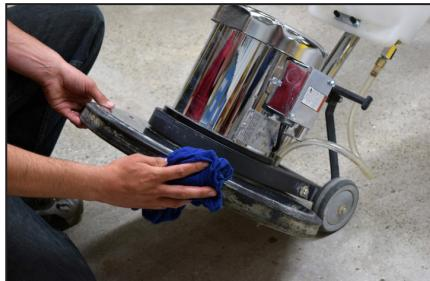
1. Clean the floor machine housing (bumper) of any residual dirt and debris. To be sure the surface is completely clean, use a clean cloth and any household cleaner or alcohol.
