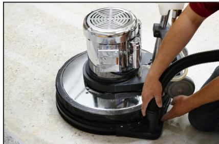
5. Attach wet/dry vacuum hose to the vacuum port of dust skirt.
