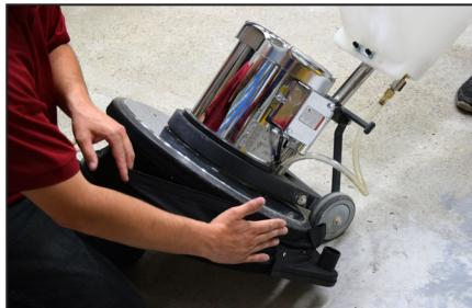
4. Apply the Malish Dust Skirt with vacuum port positioned at the bottom left of the floor machine housing when you are standing in the operator position. This will allow for maximum dust control.
