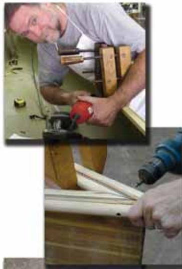
17. With the inset deck clamped in place, remove the outwale screws one at a time. Tap a deeper hole and replace each with a (well waxed) 2 or 2 1/2" screw. Your deck is now securely attached.
