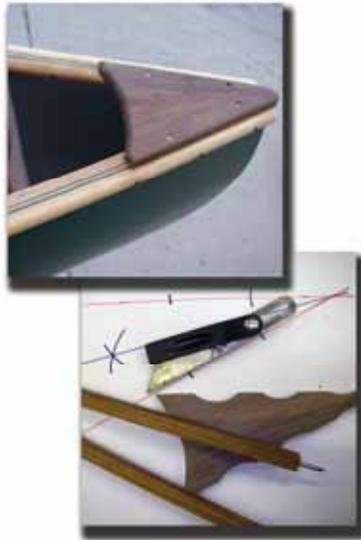
6. Repeat steps four and five to tack-in and cut the second inwale. If you're inseting the decks, your angled ends will mirror and nest inside the hull.
