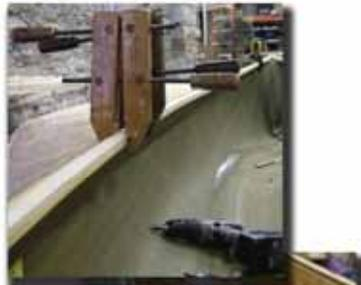
8. Clamp an outwale to the canoe placing one of the 10" screw clamps on either side of your center mark. Use a quick clamp / spring clamp near each end to support the outwale and prevent it from flopping around.
