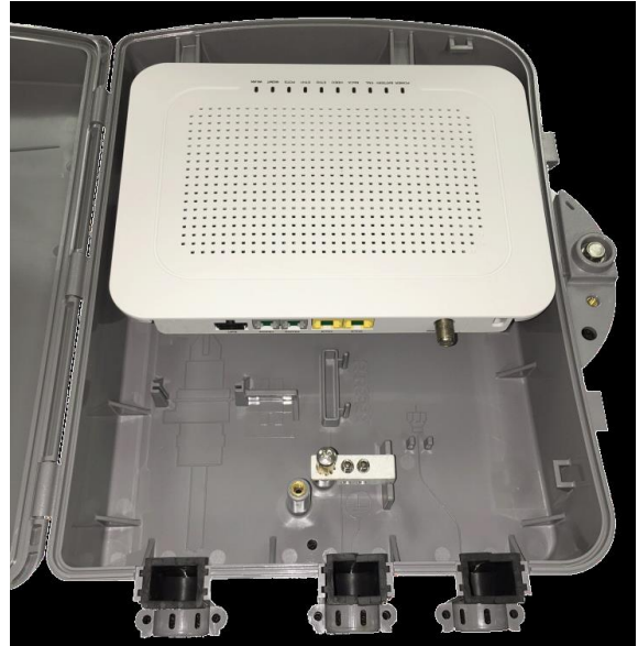
74xx ONT mounted in iPhotonix enclosure
