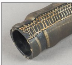
Heat Damaged Hose
