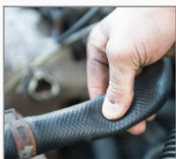
Internally Damaged Hose
