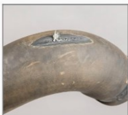
Abrasion Damaged Hose
