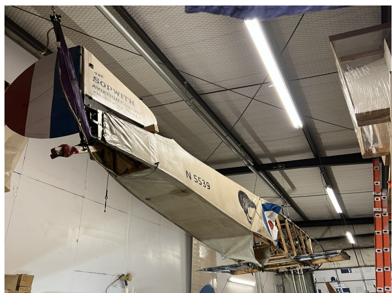
KIP fabricated, flew & crashed a 1916 Sopwith 1 1/2 strutter. The crash was the result of a design flaw in the original drawings
