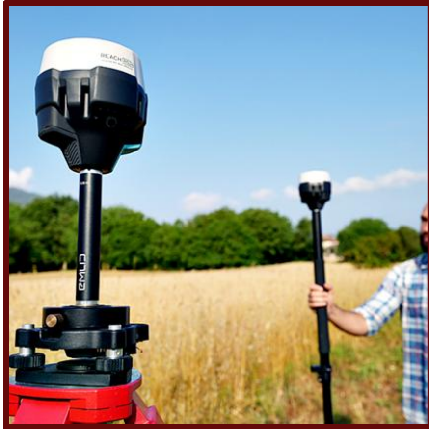
Figure 3: A base/rover pair of Emlid R2+ GNSS systems. A similar set was used on site to produce RTK level accuracy for positioning of data. Nearly the entire survey was conducted in RTK fix, which is generally around two or three inch accuracy for a system moving at pedestrian speeds.
