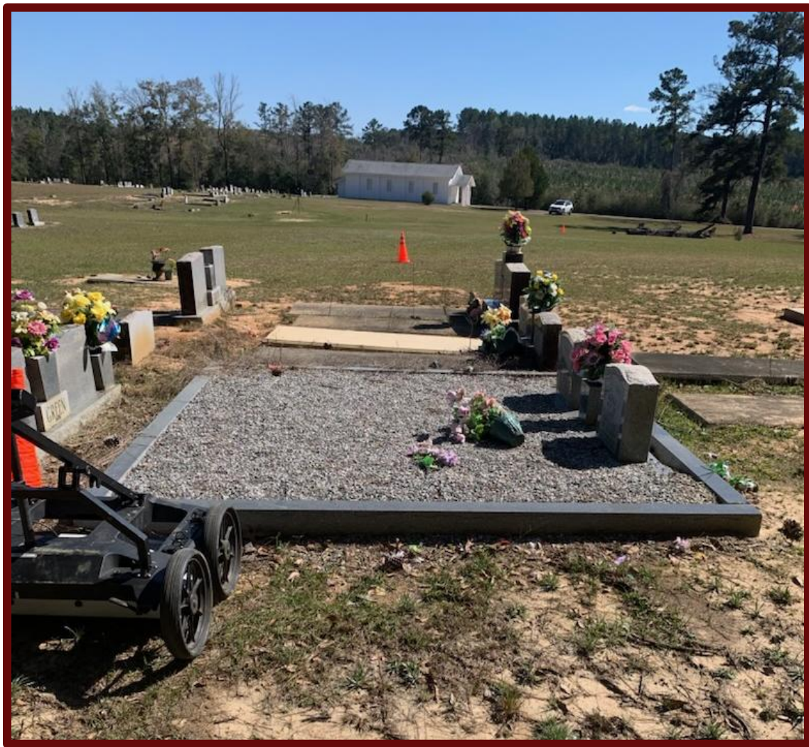
Figure 2: The Stream DP on site with road cones present for data collection purposes. GPR scanning is only possible in places where equipment can physically fit, so many holes exist within the radar survey where obstructions such as trees, headstones, and buildings prevented coverage by pedestrian equipment.
