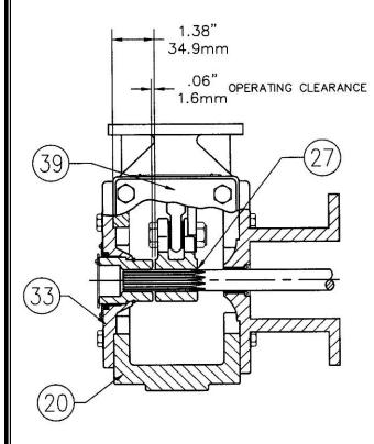
Figure 5: Lever Operating Clearance
