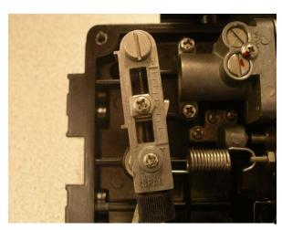
Span Adjustment - Linear
