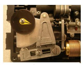
Span Adjustment - Rotary
