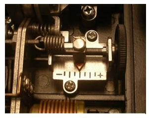
Zero Adjustment – Linear and Rotary
