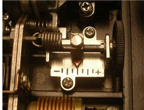
Zero Adjustment – Linear and Rotary
