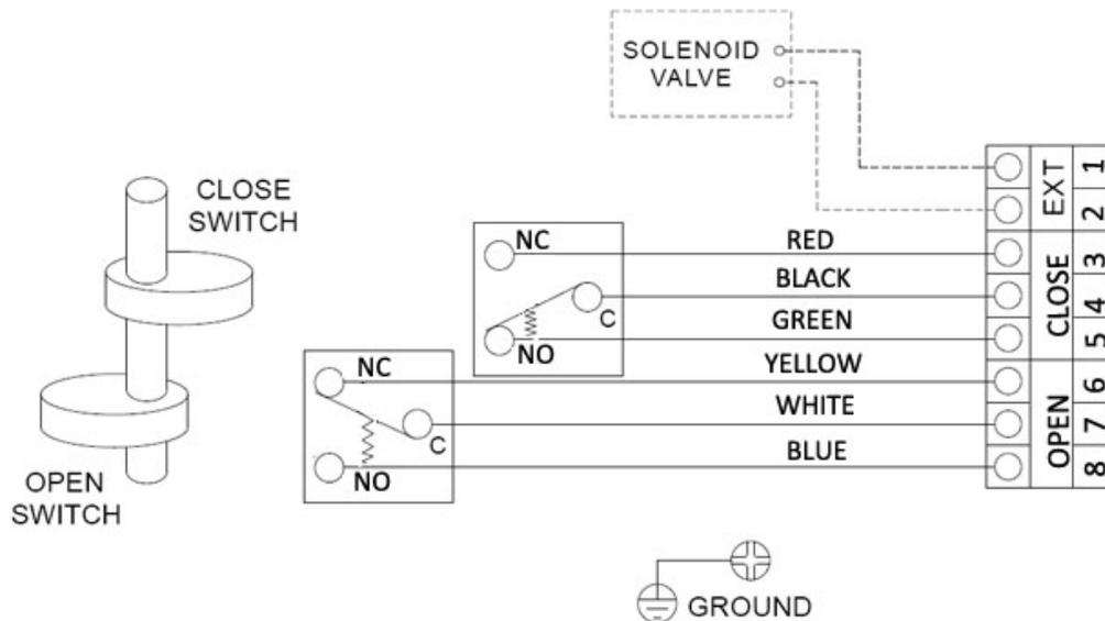
Standard CVS 500 Limit Switch is 2 Single Pole Double Throw(0.6A 125Vdc, 0.3A 250VDC, 16A 125/250VAC) and optional proximity sensors (P16AM-D3N: 8~30VDC, <=150mA or P&F sensors NJ2-V3-N: 8VDC, detected<=1mA, not detected>=3mA)
