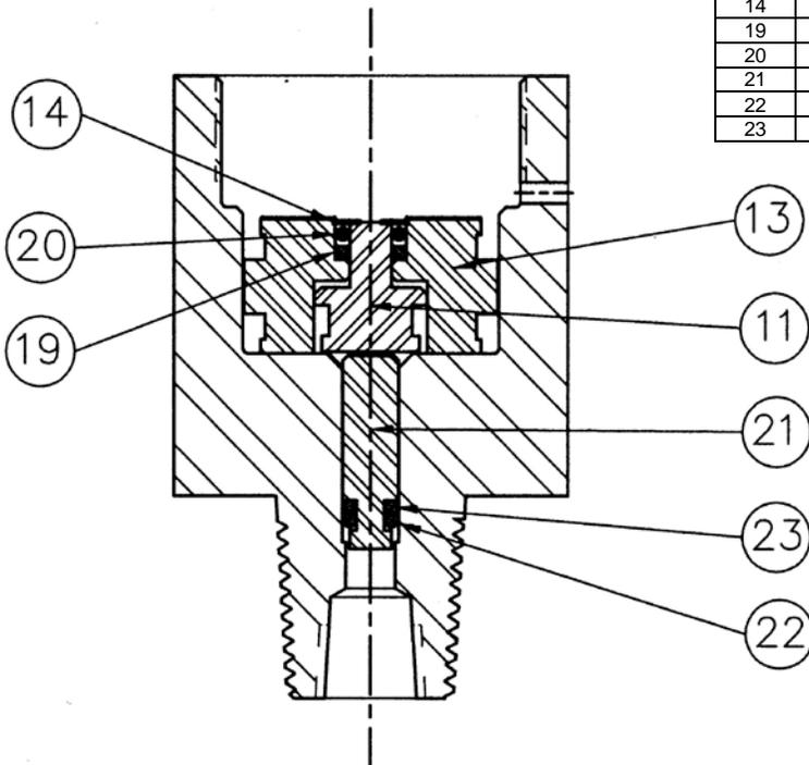
**Figure 5: 1/4" Piston Arrangement Enlarged Detail Drawing**
