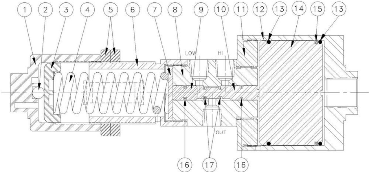
**CVS Series 7970 Low Pressure Pilot – Adjustment 2 to 15 PSI, Parts List**
