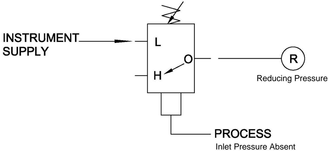
Unactuated - Monitored process control pressure has DECREASED below the Low Pressure Setting, or is absent.
