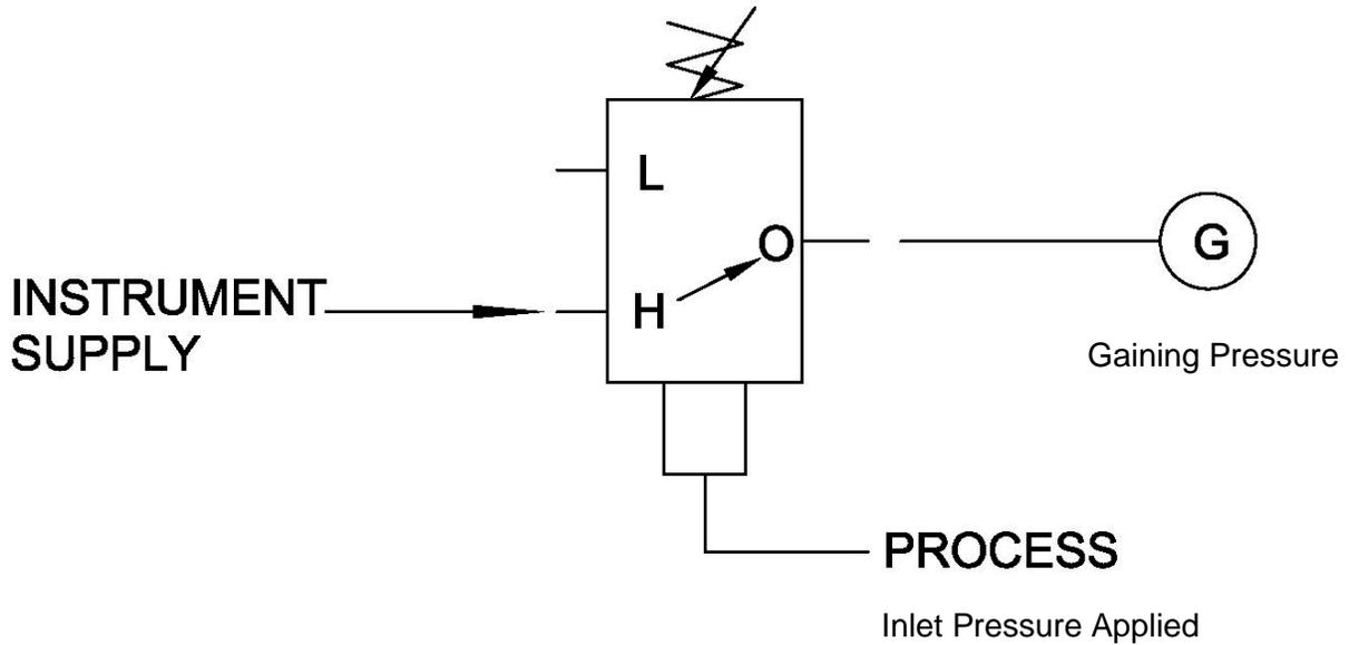
Unactuated - Monitored process control pressure is applied, but is BELOW the high pressure setting. Normal operation.
