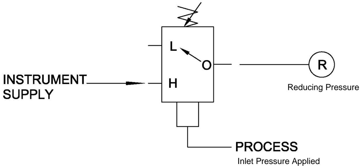
Actuated – Monitored process control pressure has INCREASED ABOVE the high pressure setting.
