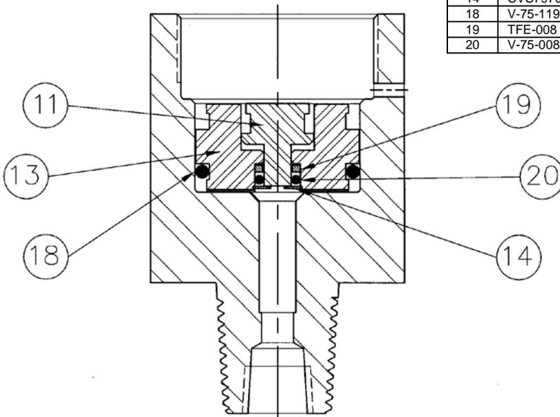
**Figure 4: 3/16 Piston Arrangement Enlarged Detail Drawing**
