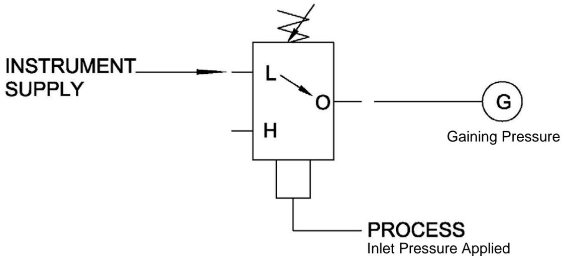
Actuated - Monitored process control pressure has INCREASED above the Low Pressure Setting. Normal operation.
