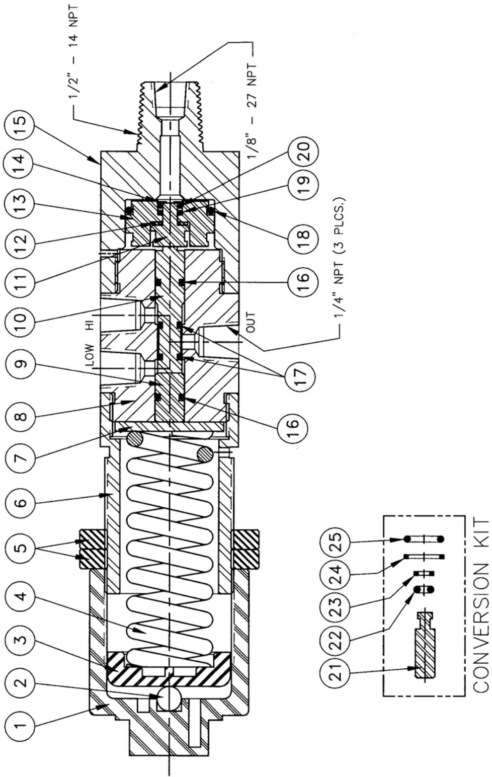
Figure 3: CVS 7970 High-Low Pressure Pilot Assembly
