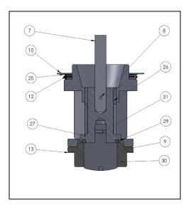
CVS Equal Percentage Valve Plug 1-1/2" & 2" Port Diameters
