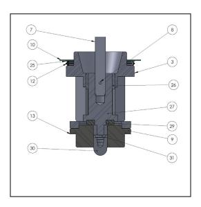
CVS M-Form Valve Plug 1/2" – 1" Port Diameters
