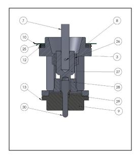
CVS M-Form Valve Plug 1/4" & 3/8" Port Diameters
