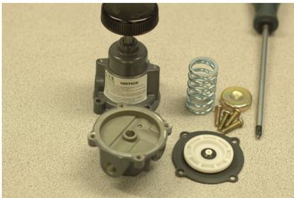
3. Remove and inspect the Diaphragm Assembly (11) from the Lower Body Assembly (1).
