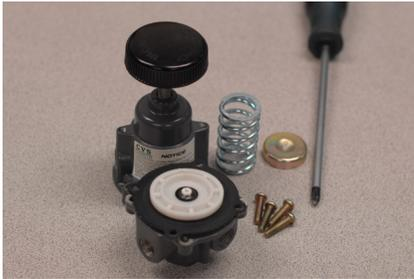
2. Remove Qty. 4, screws (17) holding the Spring Case (2) and the Body Assembly (1) together. Lift off the spring case, and remove the Spring (5), and Upper Spring Seat (6)
