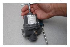
2. Remove Qty. 6, screws (18) holding the Spring Case (2) and the Body Assembly (7) together. Lift off the spring case, and remove the Spring (4), and Upper Spring Seat (3)
