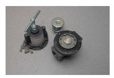
3. Unscrew the Diaphragm Assembly from the Driving Pintle (9), by first removing the Bottom Plug (12), O-Ring (13), and Pintle Spring (11). Holding the Piston Assembly (10), loosen the diaphragm assembly using a ¾" wrench or similar. Lift out the diaphragm assembly from the regulator body.
