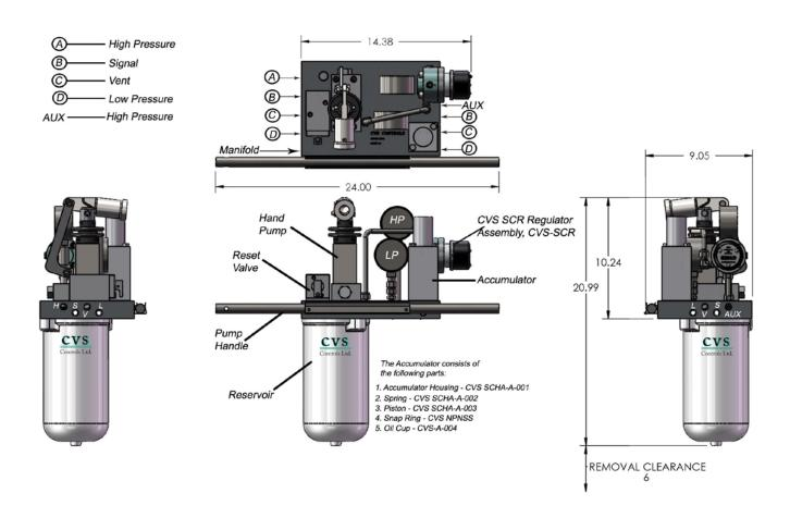
Figure 6: Self Contained Hydraulic Pump Assembly and Dimensions (in) – Low Pressure
