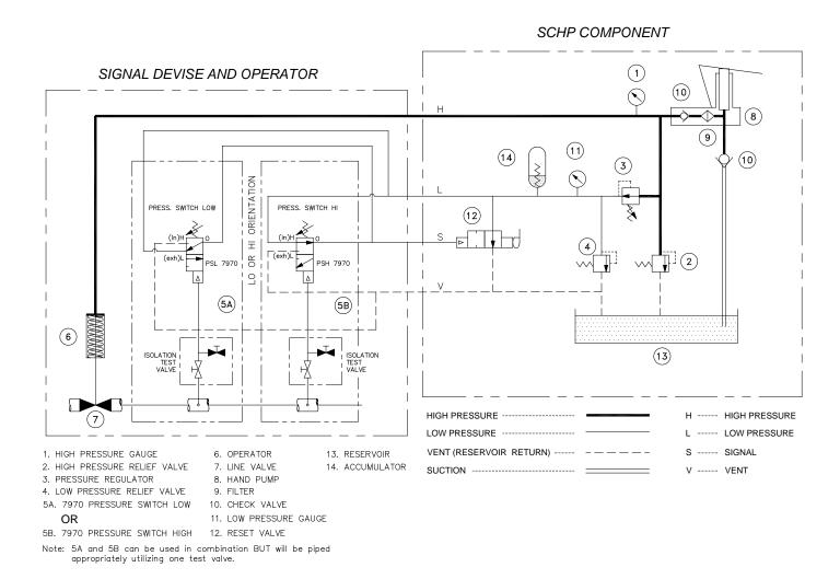
Figure 2: Module Schematic
