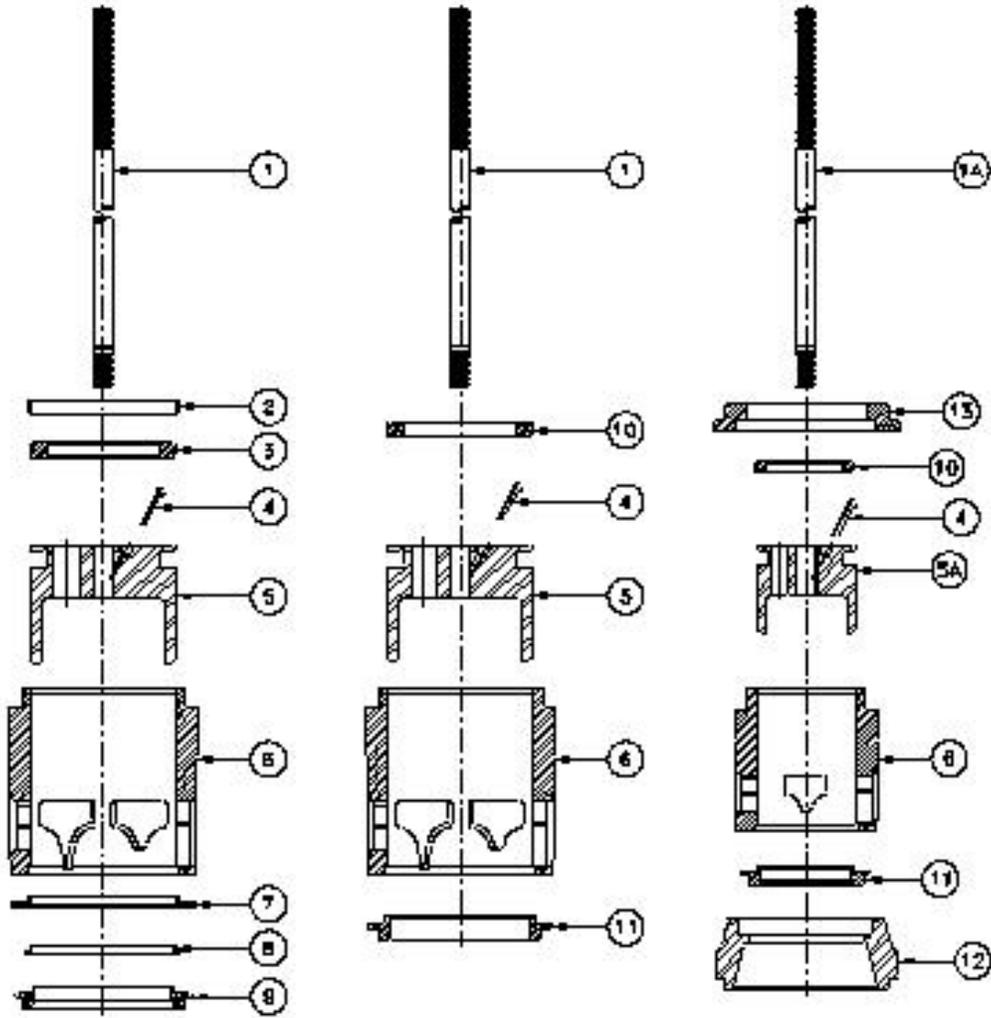
Figure 12: CVS Series E Internal Assemblies – See Following Tables
