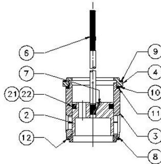
Figure 10: Trim for 1-1/2 x 1 Valve Body
