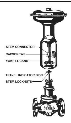
Figure 6: Actuator Mounting
