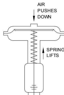
STEM MOVES UPWARD WITH LOSS OF OPERATING MEDIUM
