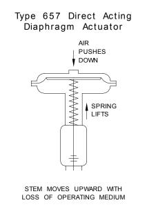
Figure 2: Schematic of CVS Type 657 Actuator
