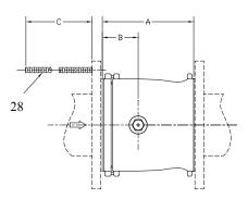
Figure 4. Required clearances for installation of design CVS V-100 Ball Valve Body
