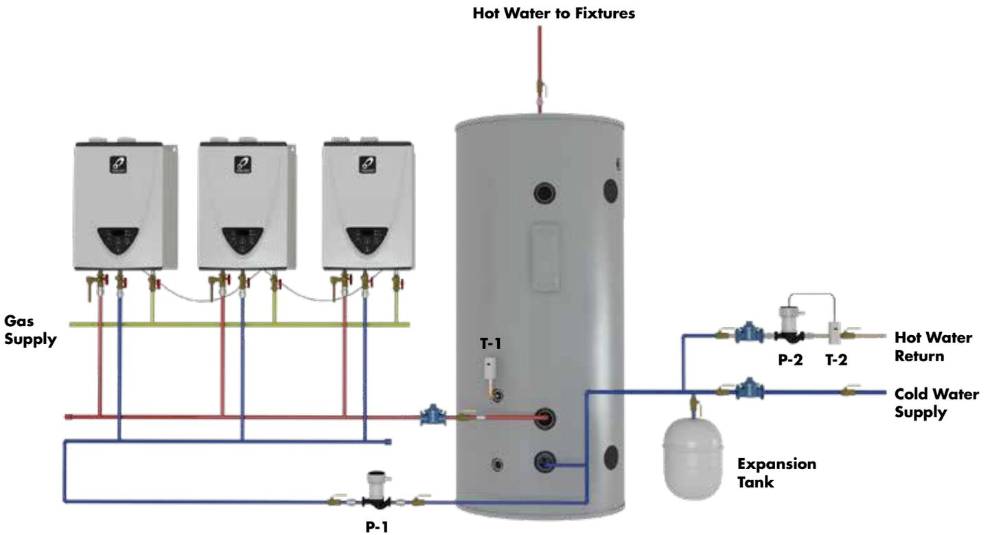
1. Tank circulation pump, P-1, should be controlled by tank aquastat, T-1.
