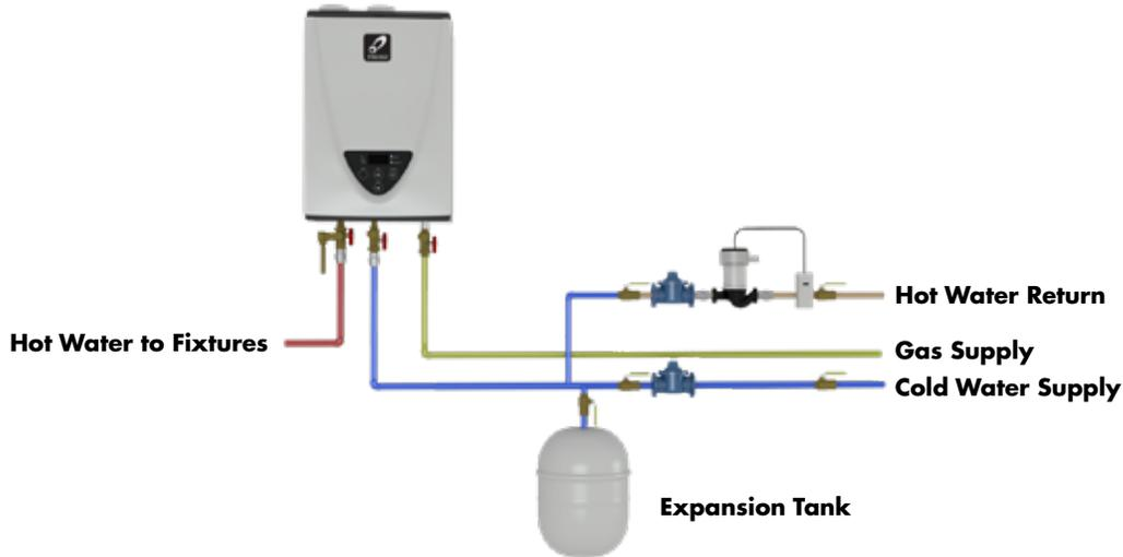
1. Recirculation pump shall be sized for 2-4 gpm per activated heater (4-8 gpm for T-M50)
