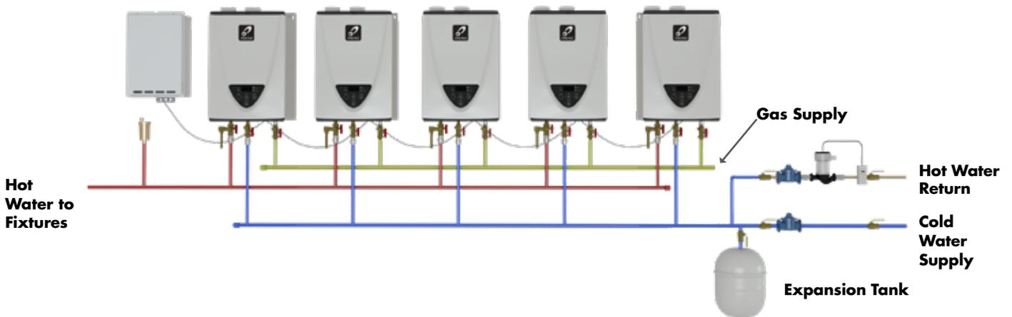
1. Recirculation pump shall be sized for 2-4 gpm per activated heater (4-8 gpm for T-M50)
