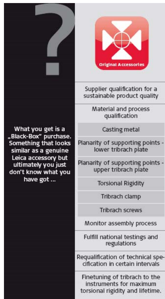
Figure 15 - Quality management steps within Leica Geosystems' tribrachs assembly
