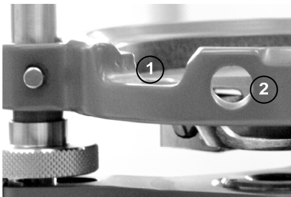
Figure 6 - Detail view of WILD GDF6 tribrach
