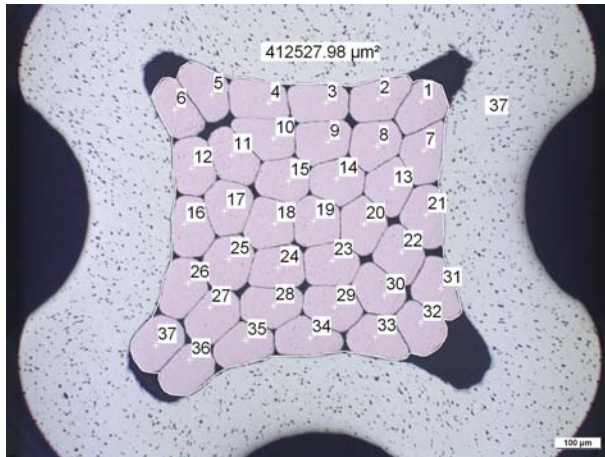
Figure 1 – cross section view of a cable crimped in connector
