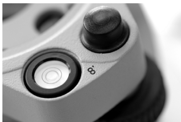
Figure 4 - Detail view of the GDF121 circular bubble
