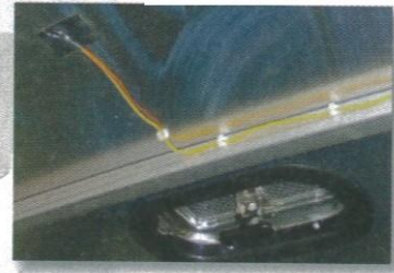
Left: Brian Jaeger, president of Innovative Green Solutions, applying Temp-Coat on H. Kent Sundling's aluminum-roofed horse trailer. inset: Wire sensors were added to test the product's cooling properties.
