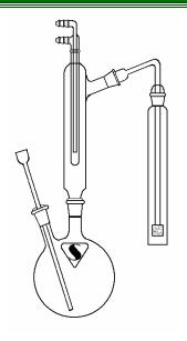
07-1000: DISTILLATION APPARATUS, CYANIDE - For use in determination of cyanide in water in accordance with ASTM D2036
